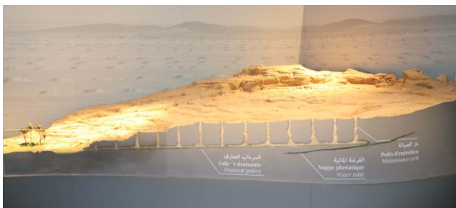
Model of khetara system at the Museum of Water Civilization Mohammed VI – ‘Aman’, Morocco
